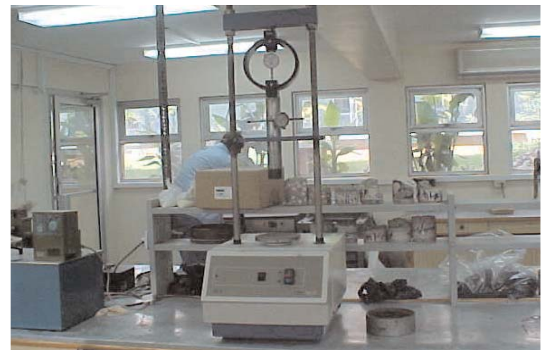
California Bearing Ratio machine, used in the lab to measure the amount of load material can withstand before deformation.
