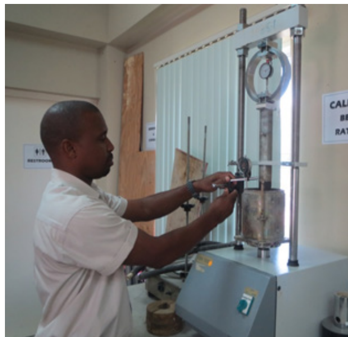
Senior Soils and Materials Technician, Glendon Brown, conducts a California Bearing Ratio Test at the Western facility.
