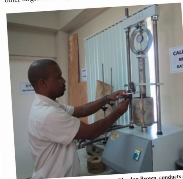
Senior Soils and Materials Technician, Glendon Brown, conducts a California Bearing Ratio Test at the Western facility.
