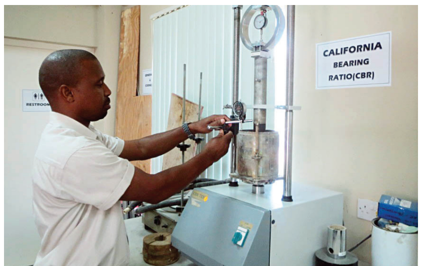
Senior Soils and Materials Technician, Glendon Brown, conducts a California Bearing Ratio Test at the Western
