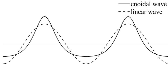
Figure 10: Comparison of profile between cnoidal wave and linear wave.
