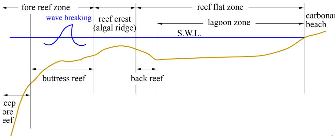
Figure 41: Cross section of coral reef
