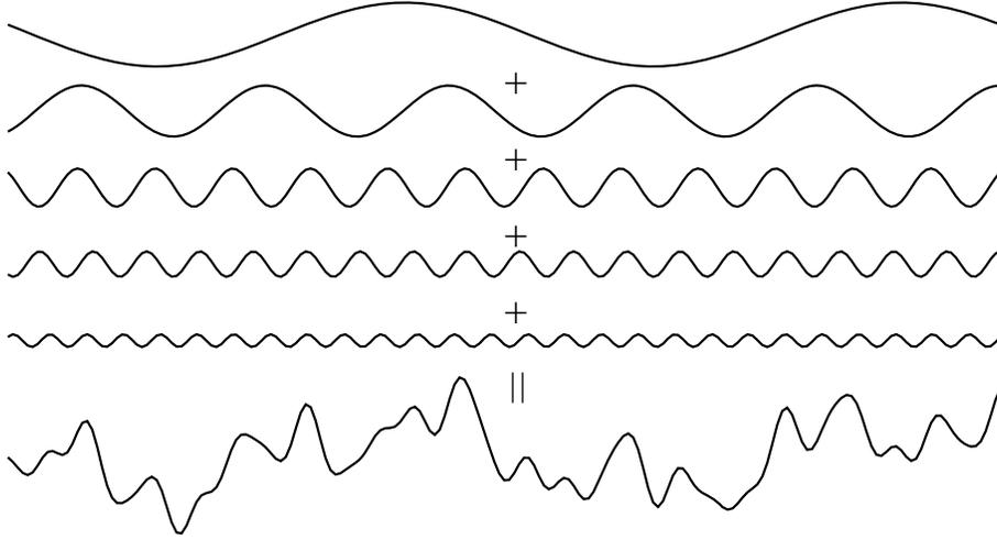
Figure 20: Superimposition of different frequency waves
