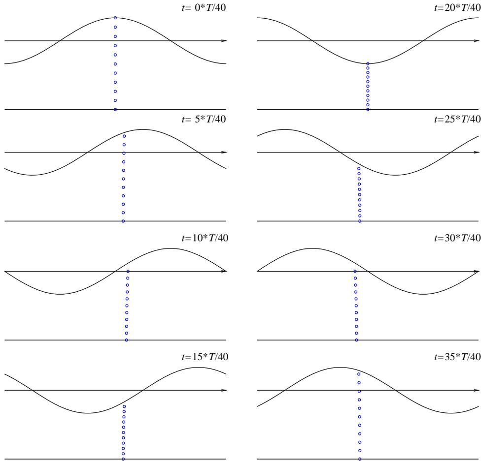
Figure 7: Orbital motion of water particles due to wave.
