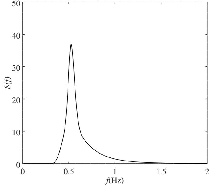
Figure 22: An example of power spectrum based on JONSWAP spectrum
