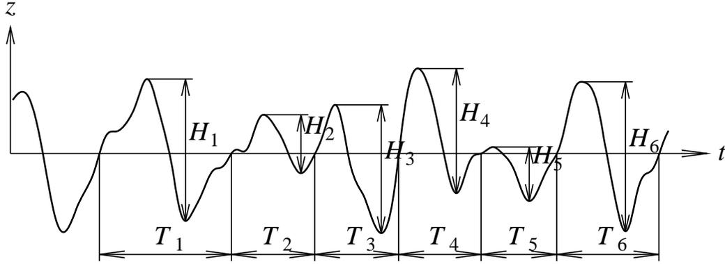
Figure 21: Wave train (wave-by-wave) analysis
