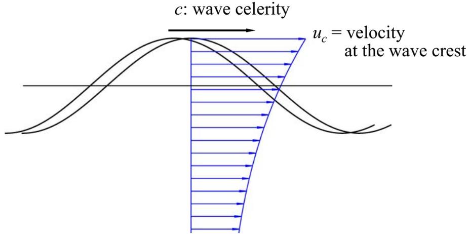
Figure 16: Definition of wave breaking with velocity at wave crest and wave celerity
