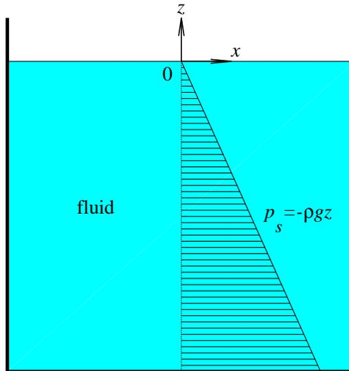
Figure 11: Hydrostatic pressure profile
