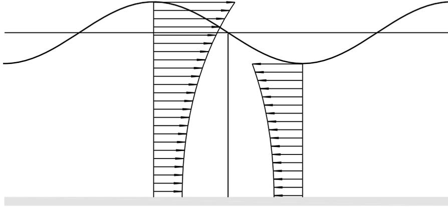
Figure 6: Velocity profile of horizontal component.
