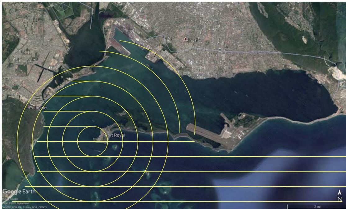
Figure 28: Schematic drawing of wave diffraction in Kingston Harbour.
