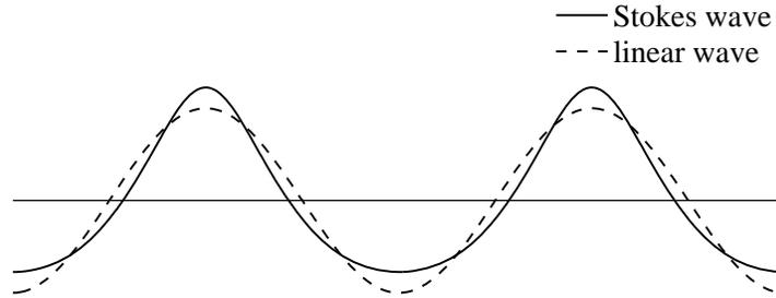
Figure 9: Comparison of profile between Stokes wave and linear wave.
