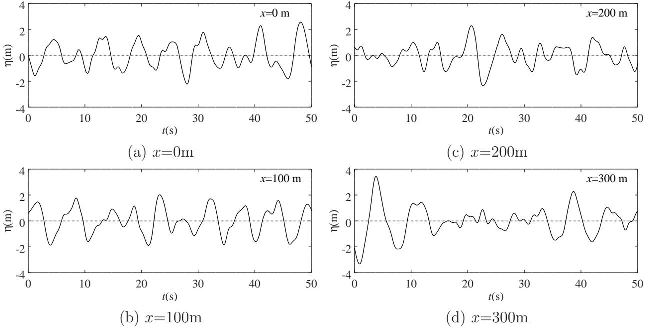
Figure 23: Time series of irregular waves at different locations while propagating.
