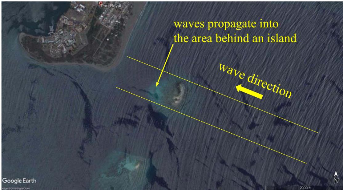
Figure 27: Wave diffraction observed behind an island near Port Royal
