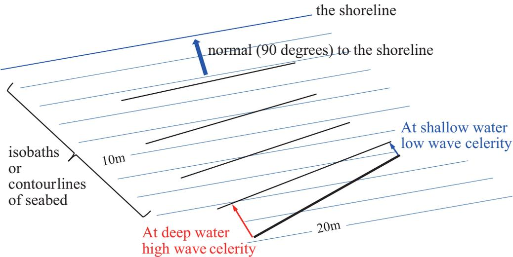
Figure 26: Mechanism of wave refraction on seabed with a uniform slope.
