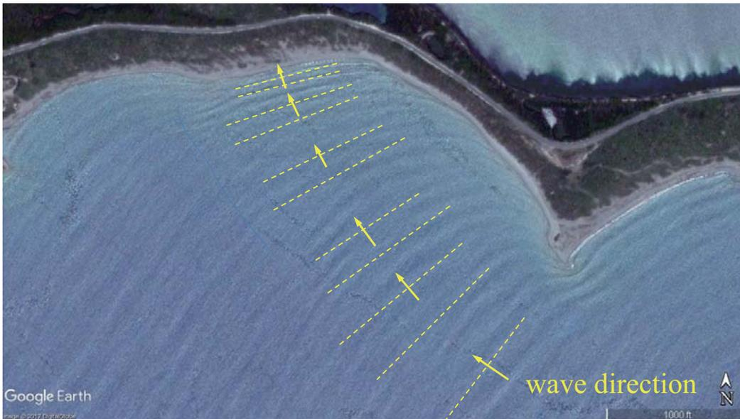
Figure 25: Wave refraction observed near Palisadoes
